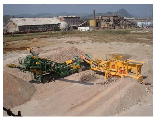
Photo 19: A typical recycling depot with crusher and screener at an industrial site on the outskirts of a city (Mitrovica, Kosovo), on hard standing and with recycled materials stockpiled ready for collection. (Source: Golder Associates).
