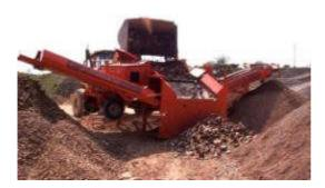
Photo 24: A primary screening feedstock for removal of soil fraction and possible contaminants (plastics, paper, non-recyclables) before crushing. (Source: Portafill)
