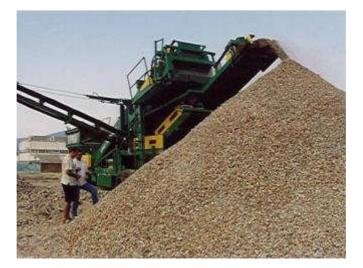
Photo 16: Recycled aggregate from crushing of building waste in Kosovo, as used for road construction or low strength concrete foundations. (Source: Golder Associates).
