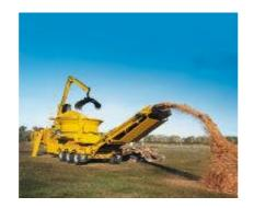
Photo 28: A typical mobile shredding plant for green wastes such as timber and wood. (Source: Vermeer)
