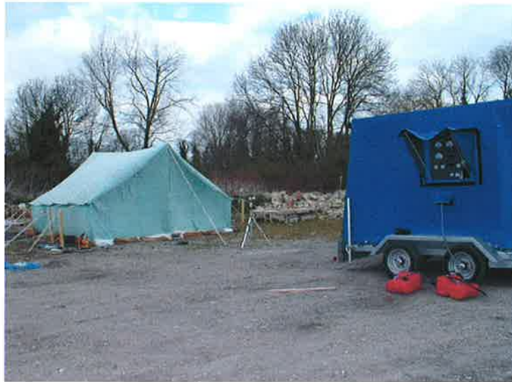
Figure 15: Tests with varying wind velocity, wind machine is shown to the right
