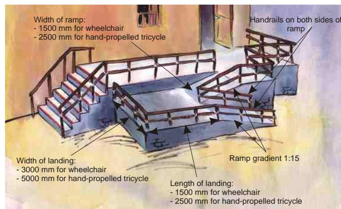
**A switchback ramp is appropriate when trying to save space and/or when the rise is higher**
