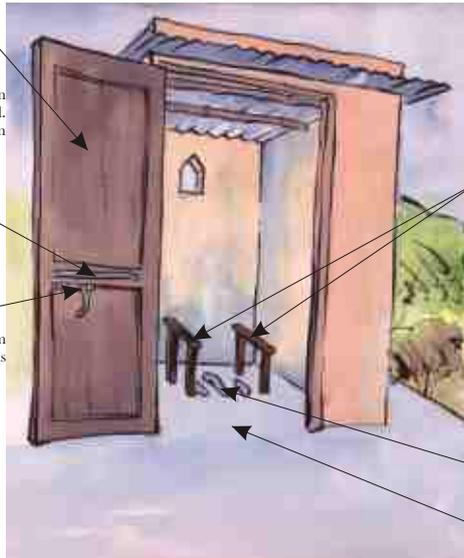
Rails should be placed on either side of the latrine and between 550 mm to 650 mm high.
