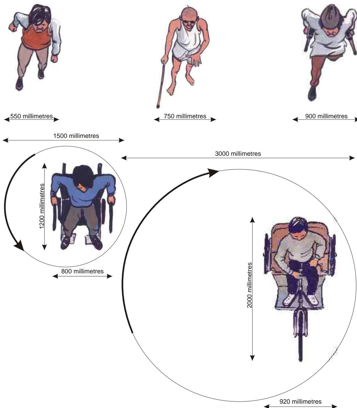
It is easier to design emergency shelters to accommodate a hand-propelled tricycle as these are the largest mobility aids and are more commonly used in villages in Nepal than wheelchairs. However, this will make aspects of the emergency shelter quite big. For example, ramp widths, turning landings and doorways will have to be wide enough to fit a hand-propelled tricycle.
