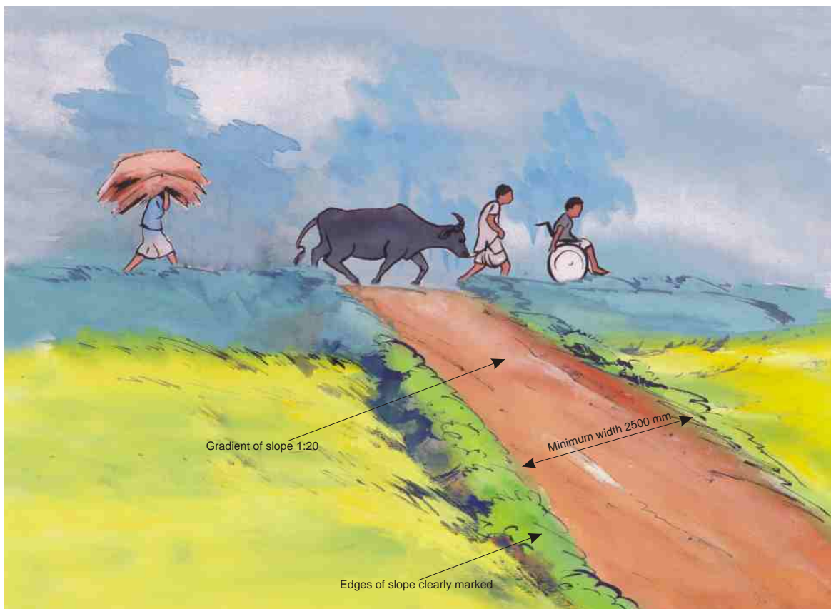
Straight slope to evacuation route
