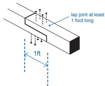
Or with a long lap joint - use a minimum of two nails for proper wood-to-wood joints and pre-drill all the timber before nailing to avoid splitting.
