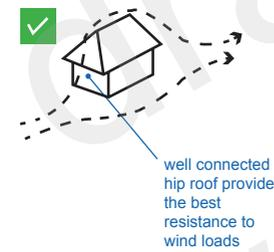
Four pitched roofs are more resistant to high wind forces than two-pitched roofs; a hip-roofed shelter with squared plan is an ideal design in hurricane prone areas.
