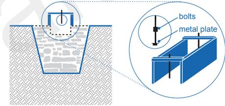
**Step 3:** pour the concrete and when it hardens, disassemble the formwork, detaching it from the tie bars. The tie bars can then be incorporated into the new wall.
